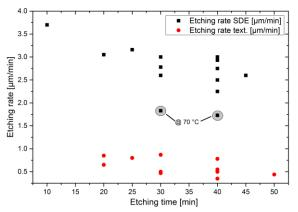
**Figure 3:** An overview over the different etching rates of all the conducted tests. Red points are indicating the etching rates of the texturing etching process while the black points are the SD-etched samples. The two highlighted points were SD-etched at 70 °C.
