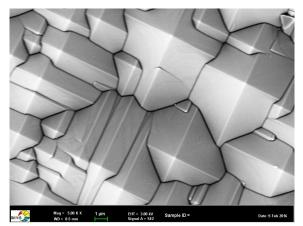
**Figure 2:** SEM pictures of well textured silicon wafers for the purpose of high efficient heterojunction solar cells. The magnification of the picture is 5000x.
