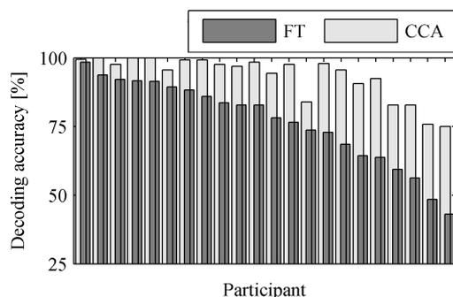
Figure 2: Single subject performance obtained in an SOV. Each of the 22 subjects shows improvement of decoding accuracy with the CCA method (light gray bars) compared to classification of FT features (dark gray bars, sorted in descending order).
