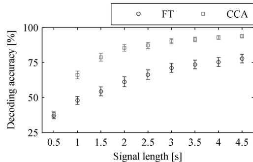
Figure 1: Dependence of decoding accuracy on signal interval length (windows of 0.5–4.5 ms width) and feature space. Average CV performance over subjects is shown. Squares represent accuracies obtained with CCA/MC classification and circles depict accuracies obtained with FT feature/rLR classification. Error bars show the standard error of the mean.
