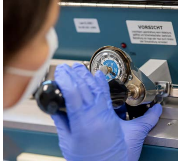
Liasan Khasanova uses a micropipette puller to prepare the tiny printing nozzles made of special glass.
