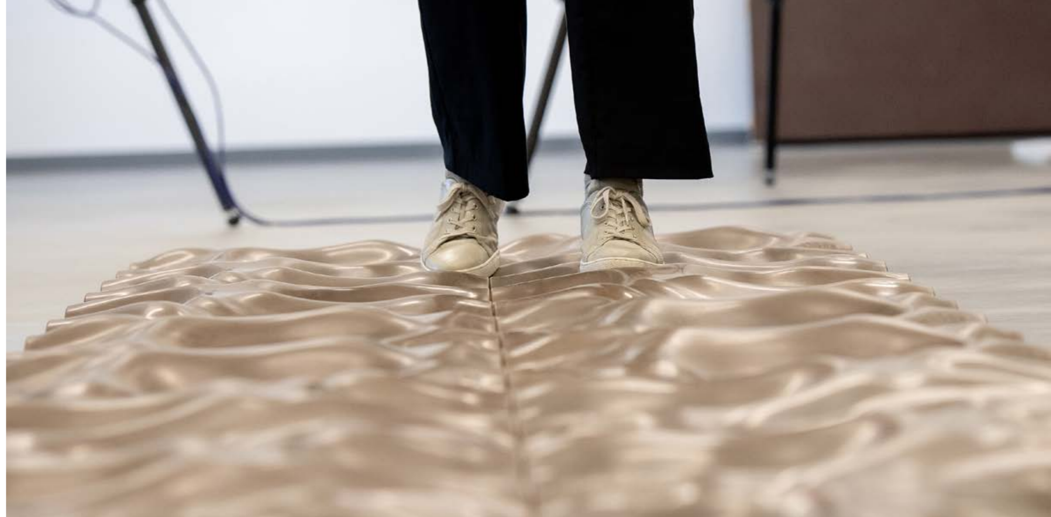
Structured floor panels simulate natural surfaces in the university's Gait Laboratory, which is jointly run by the Institute of Sports Science and the Division of Geriatrics. The panels can be used for motor training or analysis of the movement patterns that people use to compensate for surface irregularities.
