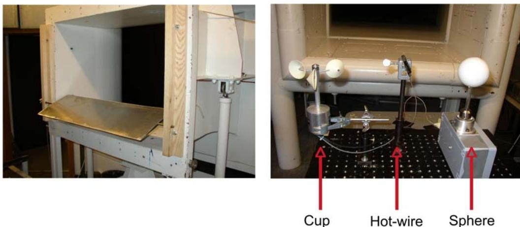
**Figure 4.** **Left:** Manually driven wind gust generator. **Right:** Position of hot-wire anemometer, cup anemometer and sphere anemometer in the wind tunnel.
