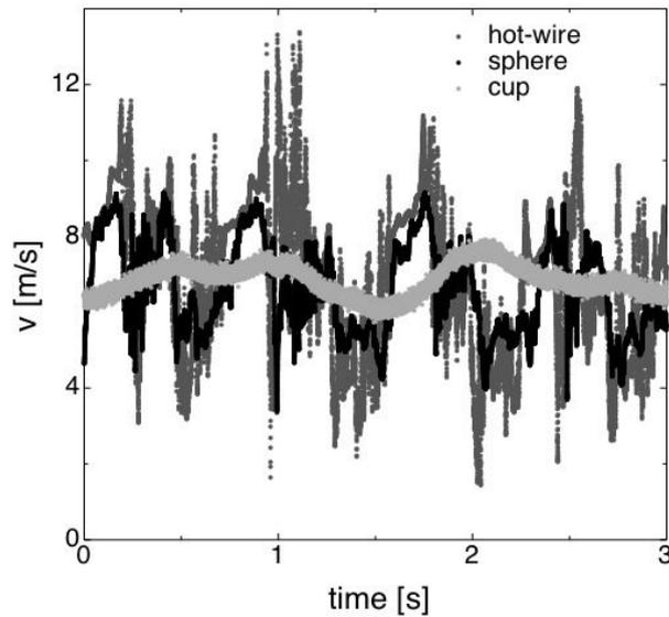
**Figure 6.** Three seconds of measured velocity for all anemometers: hot-wire (gray), sphere (black) and cup (light gray). The cup anemometer cannot follow rapid changes in the wind velocity where the sphere anemometer just misses extreme fast events.
