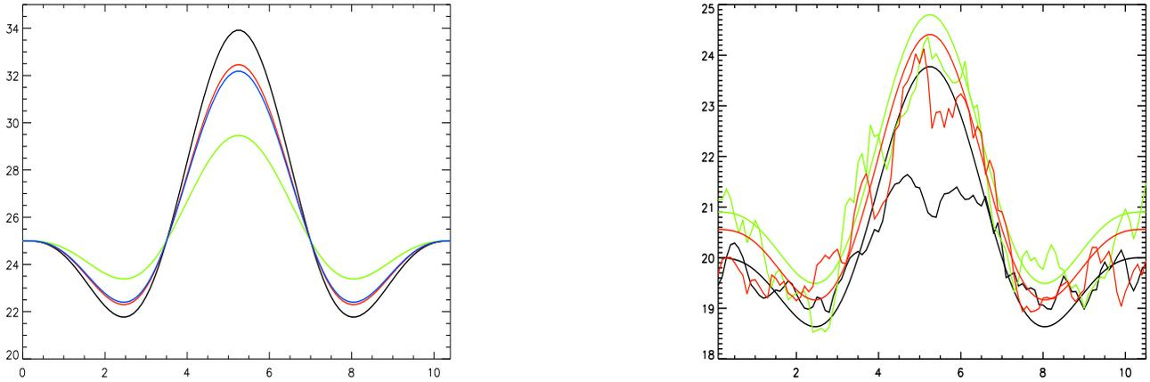
Figure 5: The EOG from the GL Offshore Guideline at site class I A (left, black), with 18% turbulence intensity, at site class I C (left, blue) with 14.5% turbulence intensity, IEC 61400-1 standard (left, red), and 9% turbulence intensity (left, green). Some examples of the EOG in December 2006 data at 80m (fluctuating line) and the EOG from the Standards with 9% turbulence intensity (smooth curve)
