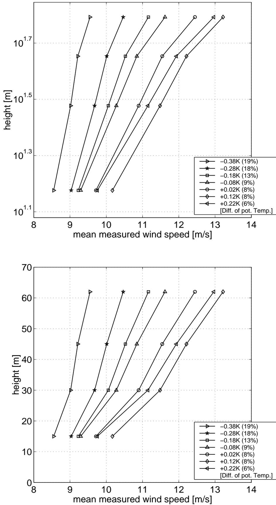
Figure 14: Sea-wind speed profiles depending on potential temperature difference  $[T55-T13+0.4K]$ . Frequency of occurrence in brackets. The wind speeds in 62m exceeding the logarithmic extrapolation seem to follow an almost linear increase. Winter period 10/2001 till 04/2002; Top: Lognormal scale, Bottom: linear scale
