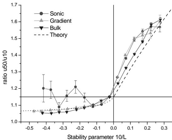
Figure 3: Bin-averaged measured wind speed  $u_{50}/u_{10}$  versus stability parameter  $10/L$  determined with three different methods
