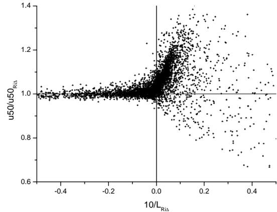
Figure 4: Ratio of measured and calculated wind speed at 50m height versus atmospheric stability; the wind speed has been calculated from the 10m wind speed using the Charnock roughness description and the stability determined via Ri number
