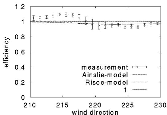
**Figure 7:** Measured and calculated efficiencies of the low WT 13. The incident wake is due to the high WT 14.
