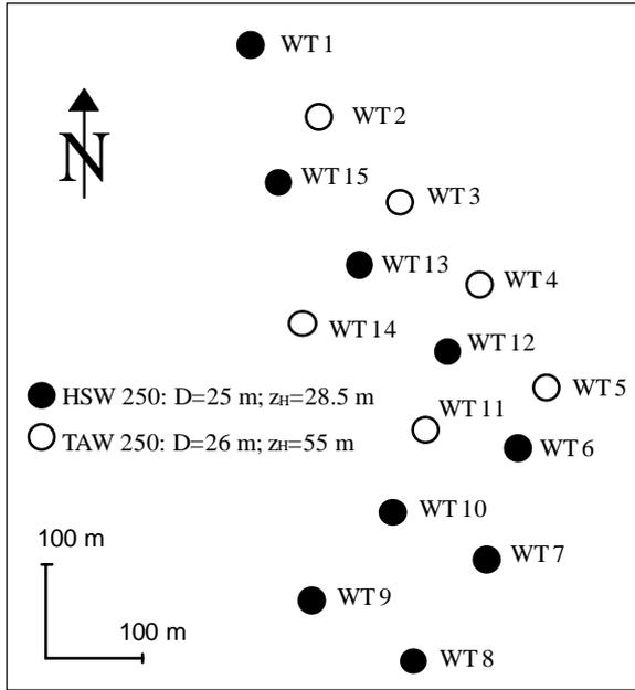
Figure 2: Geometrical set up of Husum wind farm.
