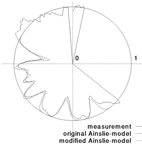
**Figure 4:** Measured and calculated (original and modified Ainslie-model) efficiencies of turbine WT 2 versus wind direction for wind speeds from 5 to 8.5 m/s. The efficiency reduction in westerly direction is due to a multiple wake. Their agreement is better for the modified model.
