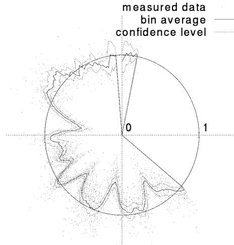
Figure 3: Measured efficiencies of turbine WT 2 of Hamswehrum wind farm versus wind direction for wind speeds from 5 to 8.5 m/s. The wake in westerly direction is a multiple wake from four turbines in a row, the other efficiency reductions are due to single wake situations.
