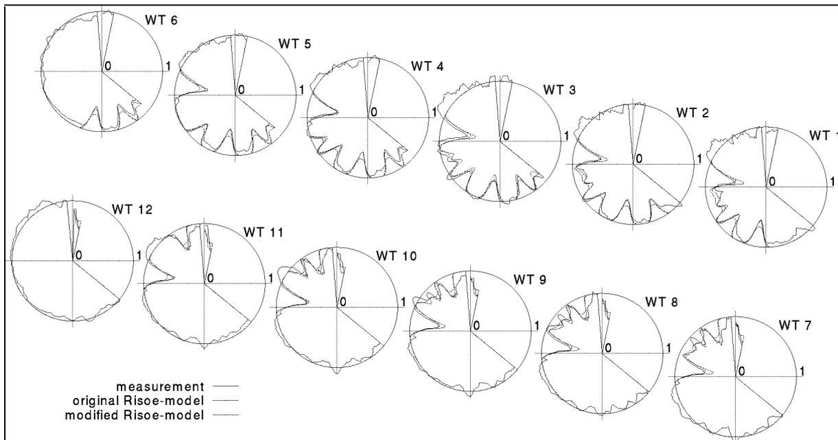
**Figure 6:** Measured and calculated (original and modified Risø-model) efficiencies of all turbines in Hamswehrum wind farm. The positions of the efficiency-curves of the turbines have been placed according to the geometrical set up of the farm. Modelling of power reductions due to single and multiple wakes is substantially better with the proposed modifications.
