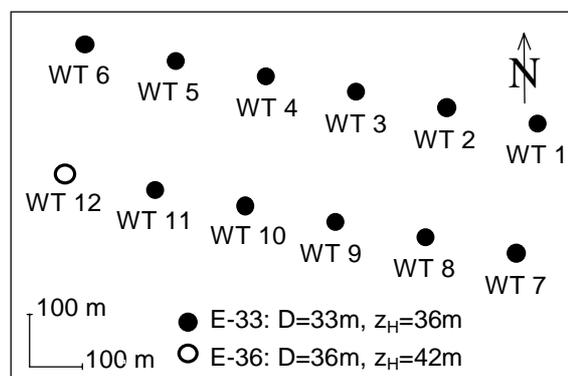
**Figure 1:** Geometrical set up of Hamswehrum wind farm (D = rotor diameter;  $z_H$  = hub height).
