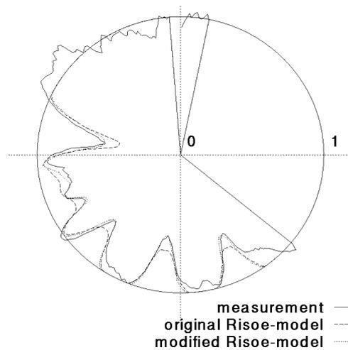
**Figure 5:** Measured and calculated (Risø-model) efficiencies of turbine WT 2 versus wind direction for wind speeds from 5 to 8.5 m/s. The original model overestimates power reductions due to the multiple wake (at 280°) and underestimates those due to single wakes. For all wakes agreement is better for the modified model.
