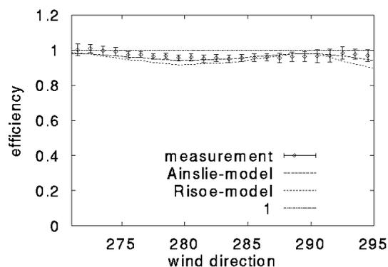
**Figure 8:** Measured and calculated efficiencies of the high WT 4. The incident wake is due to the low WT 13.
