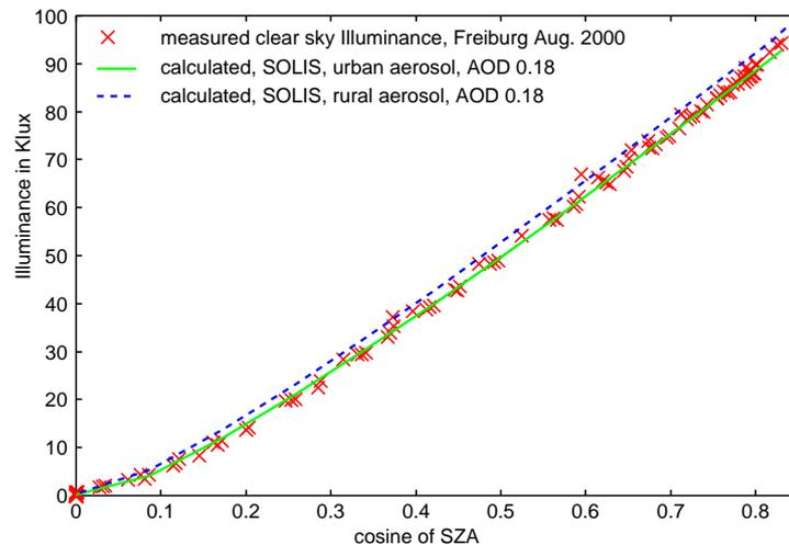
Figure 5: Measured and modelled illuminance, clear sky situations, Freiburg August 2000
