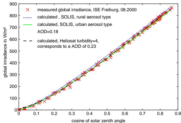
Figure 4: Comparison between SOLIS and measurements using the GADS/OPAC information for the aerosols. The calculated Heliosat clear sky irradiance is also diagrammed.
