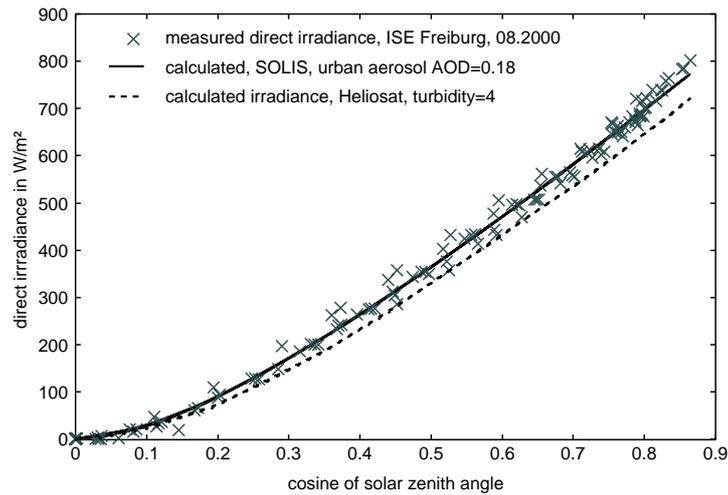
Figure 3: Comparison between SOLIS and measurements using the GADS/OPAC information for the aerosols. The calculated Heliosat clear sky irradiance is also diagrammed. The differences between the models are mainly due to the different atmospheric input information.
