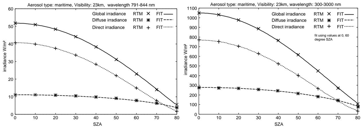
Figure 2: Comparison between RTM calculations and fit using the modified Lambert-Beer relation. Example for fit within a small wavelength band (left hand) and for a wide wavelength region (right hand)
