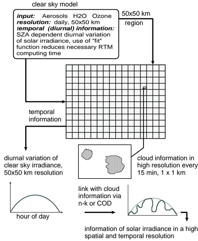
Figure 1: Diagram of the spatial and temporal linkage between clear-sky and cloud information.
