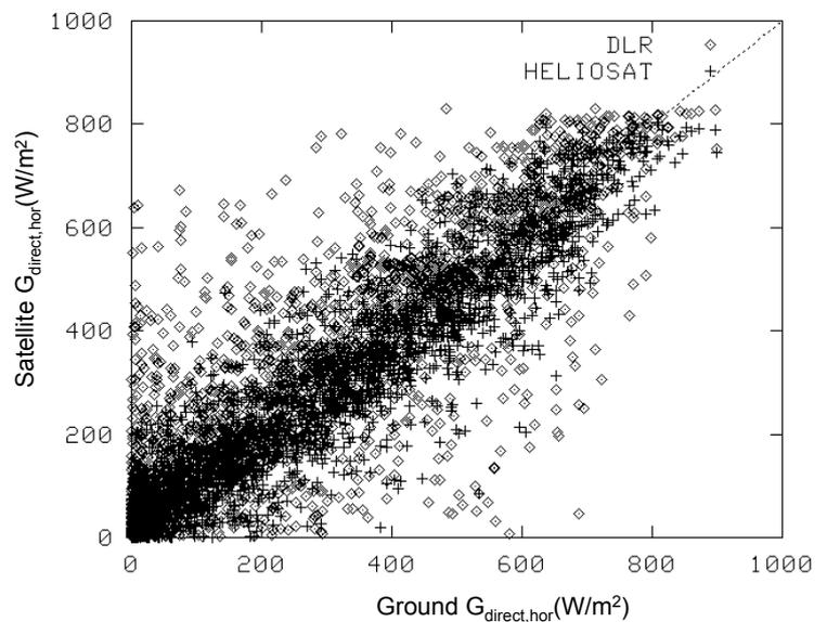
**Figure 1:** Comparison of ground measured and calculated direct horizontal irradiance, all days.
