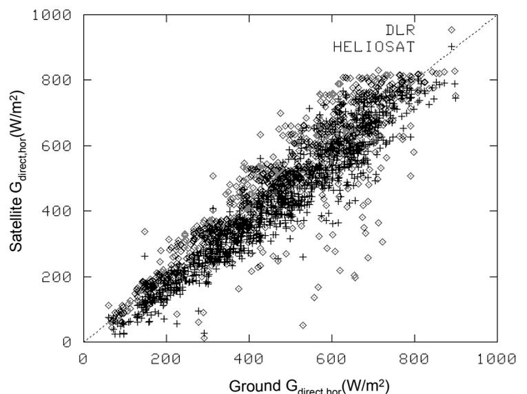
**Figure 2:** Comparison of ground measured and calculated direct horizontal irradiance. clearsky periods
