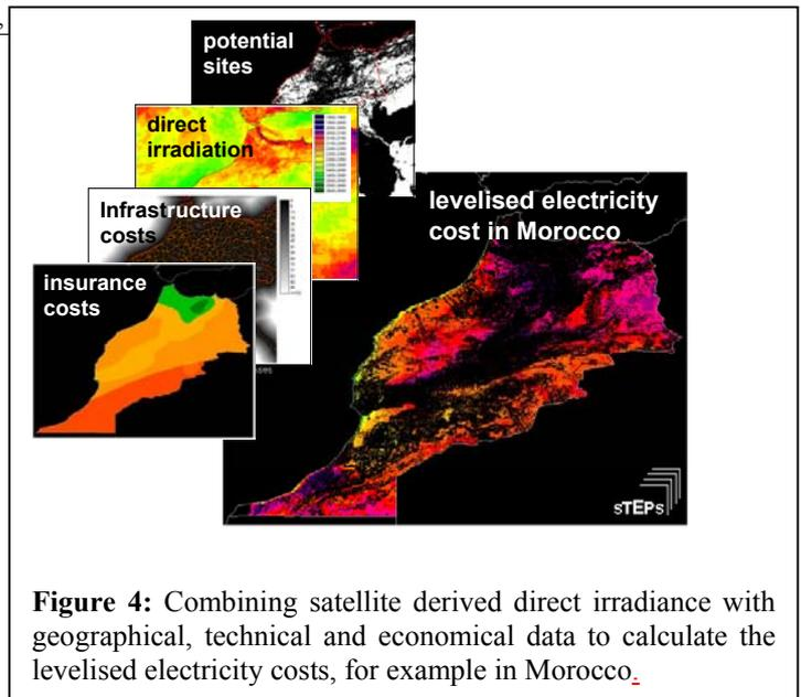
**Figure 4:** Combining satellite derived direct irradiance with geographical, technical and economical data to calculate the levelised electricity costs, for example in Morocco.
