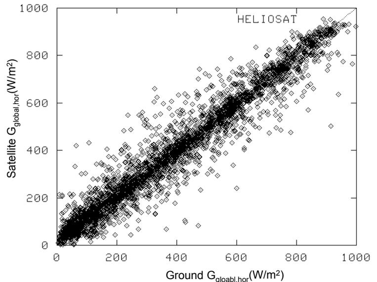
Figure 3: Comparison of global irradiance for the HELIOSAT method, all days.
