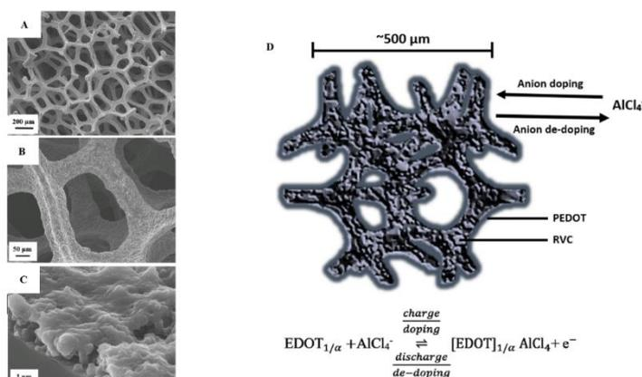
(A-C) PEDOT electro-polymerised on RVC and (D) schematic illustration of the three-dimensional RVC-PEDOT composite, which is doped (charged) and de-doped (discharged) with AlCl<sub>4</sub><sup>-</sup> anions of a chloroaluminate ionic liquid.
