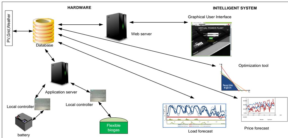
**Figure 1. Hardware and intelligent system of integrated flexible biogas-PV-battery.**
