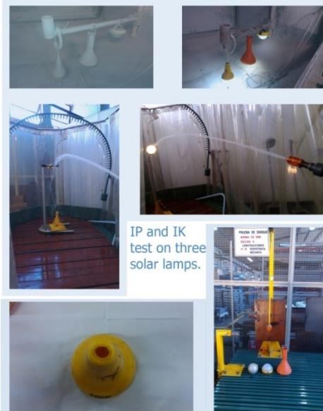
**Figure 4:** Mechanical tests on three different solar lamps (IP-IEC60598 and IK-IEC62262 test protocols)
