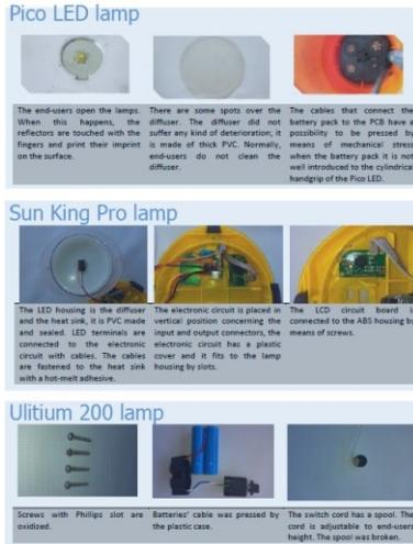
**Figure 2:** Examples of visual screening of three different solar lamps
