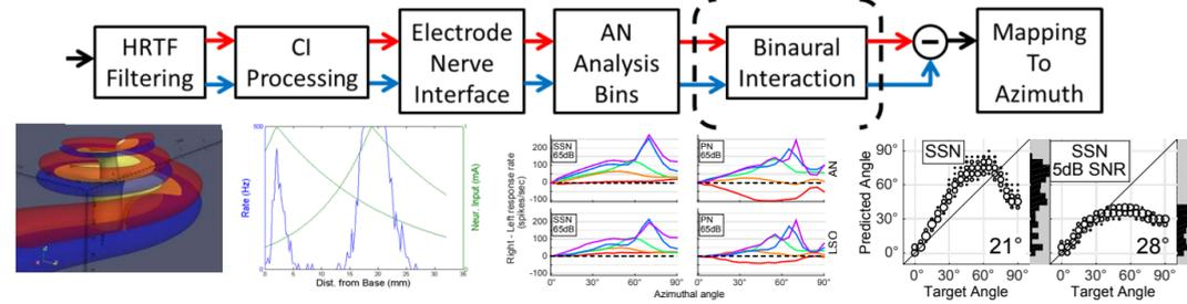
Simulation of electrical spread and neural outputs, based on relative spiking of both brain hemispheres, was performed, and neuro-inspired binaural models tested in different listening situations, including in background noise.
