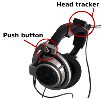
Fig. 4.2: Custom-made head tracker mounted on the headphones (Sennheiser HD800), used for perceptual evaluations in chapters 5 and 6. The push button installed on the upper right corner of the headphones enabled the listener to switch between headphone and loudspeaker presentations (see section 5.3.3).
