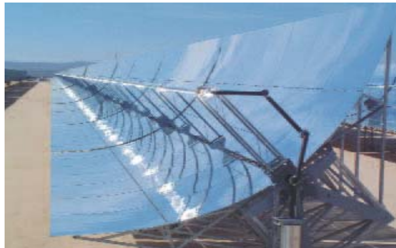
European parabolic trough collector SKALET undergoing testing at a solar power plant in Kramer Junction (USA)
