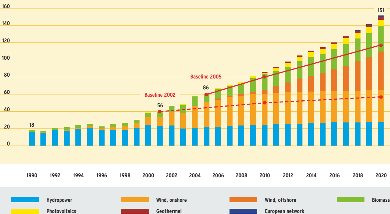
Possible development of electricity generation from renewable energy by 2020 with the EEG in effect
