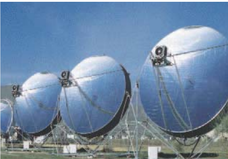
Parabolic-dish power plants ("Dish system") with a Stirling motor generator undergoing testing and demonstration operation at the Plataforma de Almeria, Spain: up to 30 % solar-electric efficiency is achieved with these systems.
