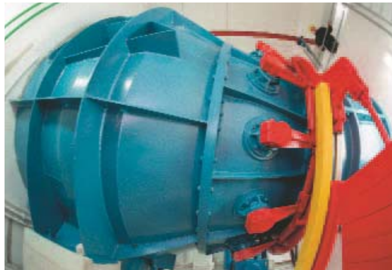
This water turbine system in Cottbus has a capacity of 280 kW.
