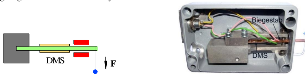
Fig. 1: Left: Principle of force measurement using a bending rod (green) fixated on the left by a block (gray). The gravitational force \mathbf{F} = \mathbf{G} of a suspended weight (blue) causes a deformation of the staff which is measured by the strain gauge (SG, yellow). The mechanical limits (red) prevent overstraining the rod by excessive forces. Right: View into the casing of a force sensor used in this laboratory course. The strain gauges glued to the rod are very thin and barely visible. The cables are the connections of the SG. They run to the connecting terminal on the top left to which the measuring amplifier is connected.
