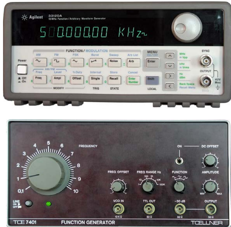
Fig. 4: Front views of two function generators used in the laboratory. Top : AGILENT 33120A, bottom : TOELLNER 7401. At the FG TOELLNER the frequency of the output signal is the product of the value adjusted at the switch FREQ RANGE (in this case 100 Hz) and the multiplier adjusted at the rotary knob FREQUENCY (1 Hz). At the represented setting therefore f = 1 \times 100 \text{ Hz} = 100 \text{ Hz} .
