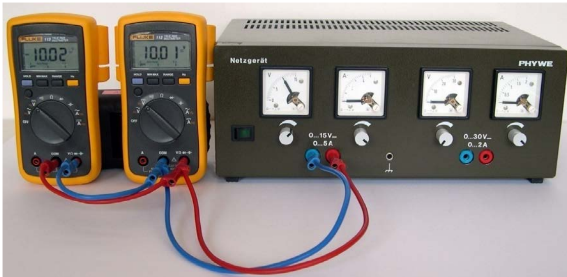
Fig. 2: On the polarity of the voltage from a power supply. At the left output a voltage of approx. 10 V is adjusted. The left multimeter (type FLUKE) reads a voltage of - 10.02 V, the right one reads a voltage of + 10.01 V 3 . Reason: The reference point for measuring the voltage (black terminal COM at the multimeter) is connected with the red terminal of the power supply (the one with the higher potential) on the left side and with the blue terminal (the one with the lower potential) on the right side.
