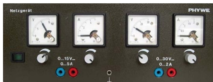
Fig. 1: Power supply of the type PHYWE. At both outputs (red and blue terminal) a voltage of approx. 10 V is adjusted.
