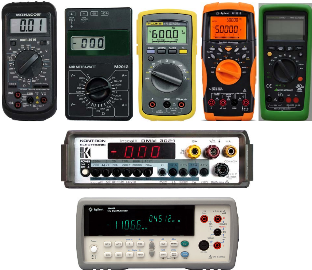
Fig. 5: Front views of seven multimeters used in the laboratory. Top from left to right: MONACOR DMT-3010, ABB METRAWATT M2012, FLUKE 112, AGILENT U1251B, METRALINE DM 62; centre : KONTRON DMM 3021; bottom : AGILENT 34405A.
