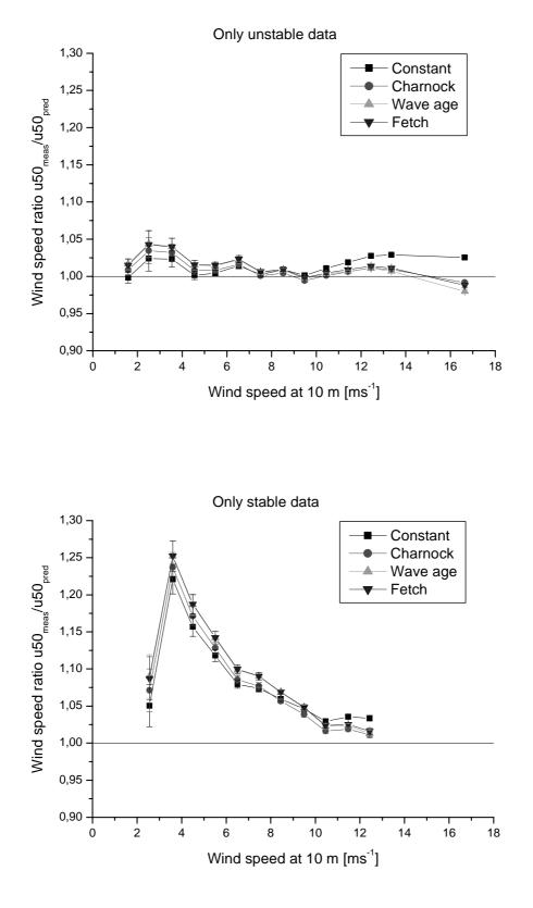
Figure 5: Bin-averaged ratio of measured and predicted 50 m wind speed versus wind speed at 10 m height with L determined by the bulk method and  $z_0$  modelled with four different models (see text)
