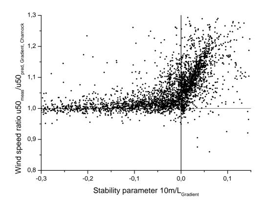
Figure 2: Deviation R between measured and predicted 50 m wind speeds versus 10m/L; L derived with the gradient method and  $z_0$  with the Charnock model
