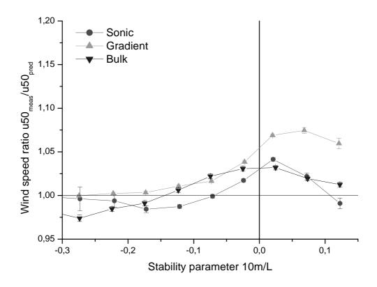
Figure 8: Bin-averaged ratio of measured and predicted 50 m wind speed versus stability parameter 10m/L with L determined by the sonic, gradient and bulk methods and  $z_0$  with Charnock model; the proposed correction method for thermal influences is used
