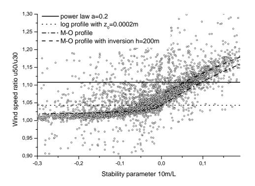
Figure 16: Wind speed ratio between 50 m and 30 m height measured at Rødsand versus atmospheric stability; also shown are calculations with different wind speed profiles (see Figure 15)
