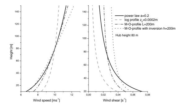
Figure 15: Comparison of wind speed (left) and wind shear (right) height profiles for different profile forms; the wind speed at hub height 80 m is 10 ms<sup>-1</sup>; shown are a power law profile with a=0.2, a logarithmic profile with  $z_0=0.0002m$ , a Monin-Obukhov profile with  $z_0=0.0002m$  and L=200 m, and a profile with inversion layer correction from eq. (16) with  $z_0=0.0002m$ , L=200 m and h=200m
