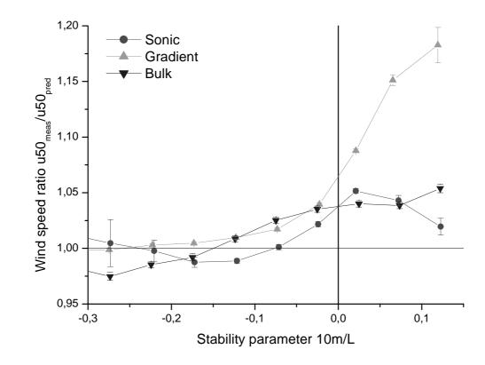
Figure 3: Bin-averaged ratio R of measured and predicted 50 m wind speed versus stability parameter 10m/L with L determined by the sonic, gradient and bulk methods and  $z_0$  with Charnock model
