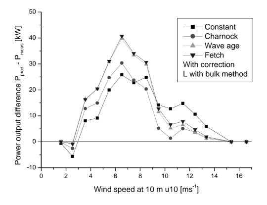
*Figure 13: Difference between predicted and measured power output, bin averaged for 10 m wind speed; Comparison of different models with wind profile correction*
