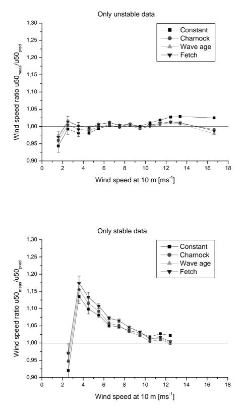
Figure 9: Bin-averaged ratio of measured and predicted 50 m wind speed versus wind speed at 10 m height with L determined by the bulk method and  $z_0$  modelled with four different models (see text); the proposed correction method for thermal influences is used
