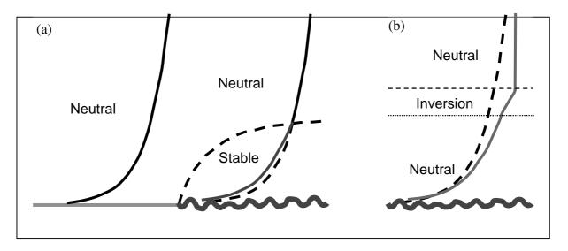
Figure 6: Conceptual sketch of the flow regime with warm air advection over colder sea. The wind profile is shown compared with a neutral profile.
