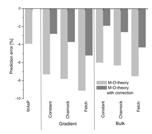
Figure 14: Relative error in power output prediction  $(P_{meas}-P_{pred})/P_{meas}$  of an example turbine for the 2 year long Rødsand data set; different methods to extrapolate the wind speed measurement at 10 m height to 50 m are used (see text); the result with the WAsP method is also shown
