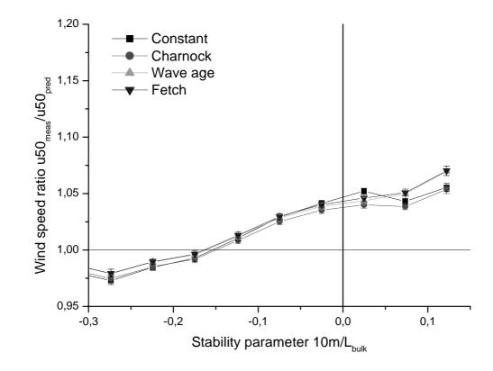
Figure 4: Bin-averaged ratio of measured and predicted 50 m wind speed versus stability parameter 10m/L with L determined by the bulk method and  $z_0$  modelled with four different models (see text)
