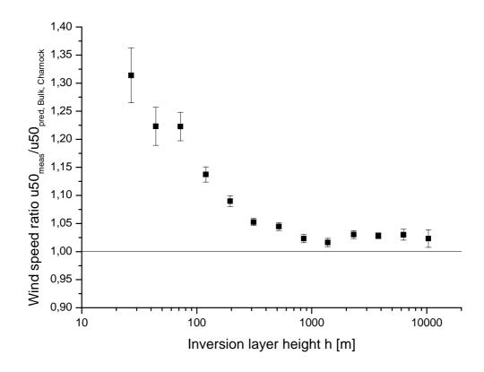
Figure 7: Deviation R bin averaged for the estimated height of inversion layer h (from eq. (15)); When estimating  $u50_{pred}$ , the bulk method has been used to determine L and the Charnock equation for the estimation of  $z_0$
