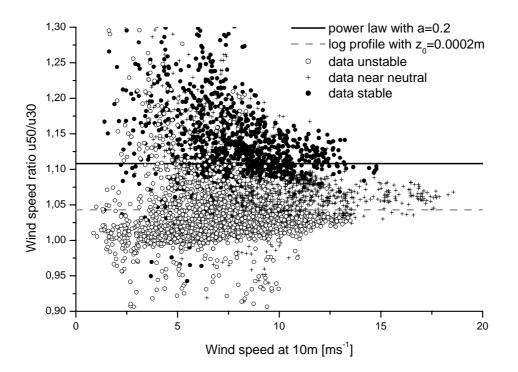
Figure 17: Wind speed ratio between 50 m and 30 m height measured at Rødsand versus wind speed at 10 m height for different stability classes (10m/L<-0.05 unstable, -0.05<10m/L<0.05 near-neutral, 10m/L>0.05 stable stratification); also shown are calculations with different wind speed profiles (see Figure 15)
