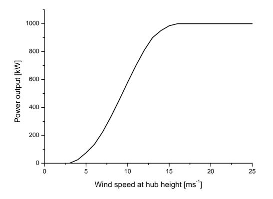
Figure 10: Power curve of the example wind turbine
