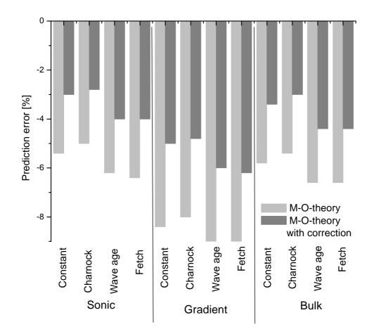
Figure 11: Error in power output prediction  $(P_{meas}-P_{pred})/P_{meas}$  of an example turbine for the Rødsand data set; different methods to extrapolate the wind speed measurement at 10 m height to 50 m are used (see text)
