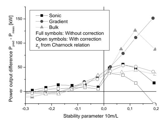
Figure 12: Difference between predicted and measured power output, bin averaged for stability parameter 10m/L; L derived with Sonic, Gradient and Bulk methods; Prediction with and without wind profile correction
