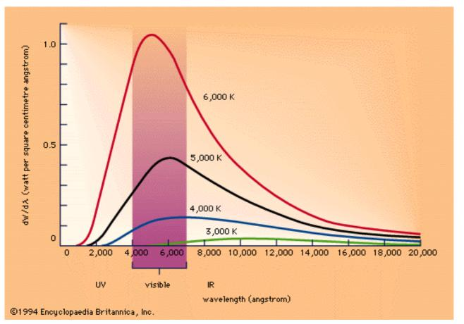
Electromagnetic energy dWemitted per unit area and per second into a wavelength interval,  $d\lambda = 1$  Å, by a blackbody at various temperatures between 3000 and 6000 K as a function of wavelength.
