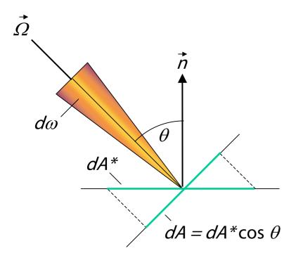
According to the cosine law, the radiance crossing a surface  $dA^*$ , whose normal n makes an angle  $\theta$  with the beam axis  $\Omega$ , is:
