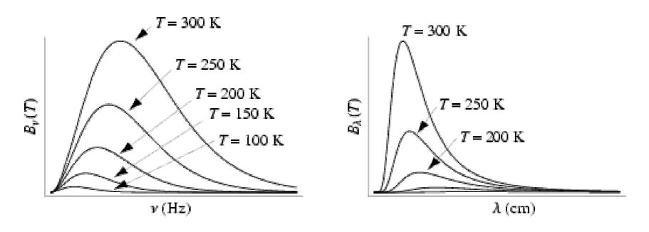
Intensity radiated by a blackbody as a function of frequency (left) or wavelength (right)
