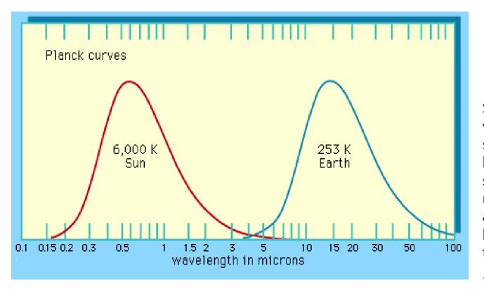
Spectrum of the Earth as viewed from space showing distinction between reflected sunlight and planetary radiation. The Earth is assumed to emit as a blackbody at an average temperature of 253 K. *Royal Meteorological Society.*
