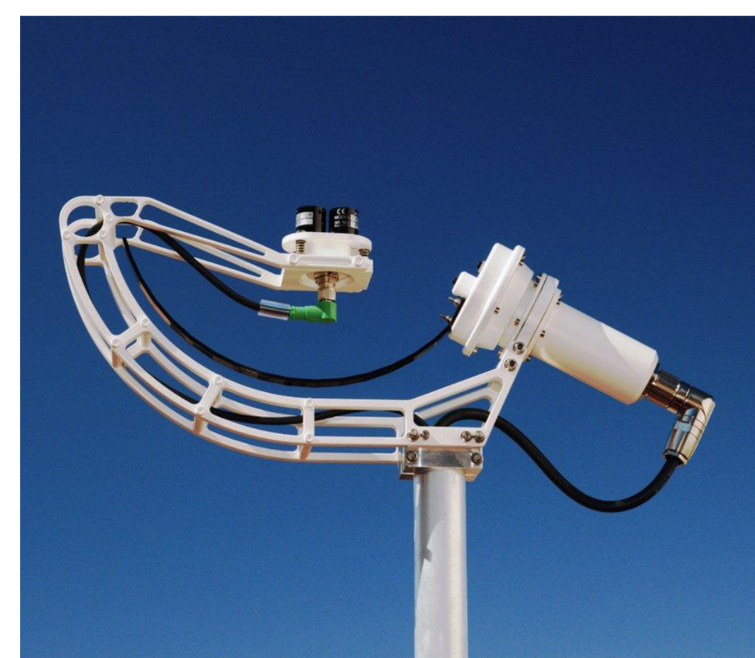
Fig. 2: RSI sensor in rest position
