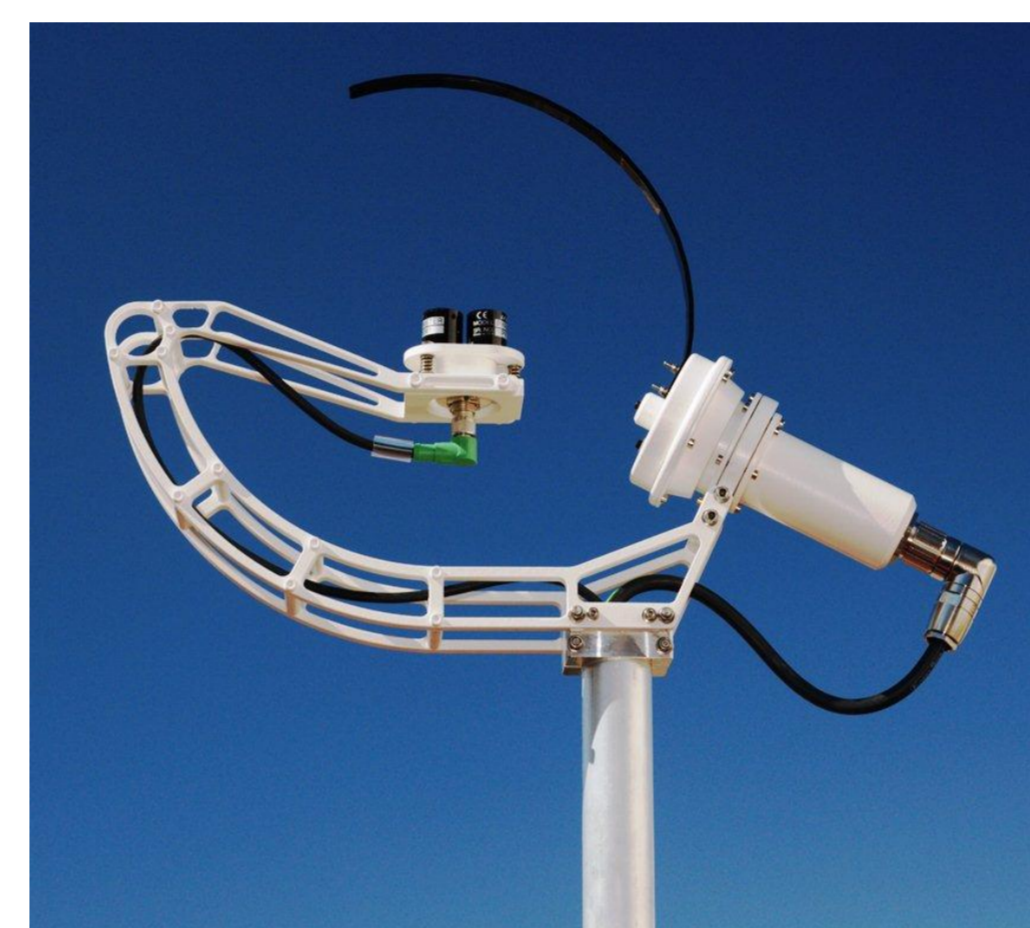
Fig. 3: RSI sensor during rotation
