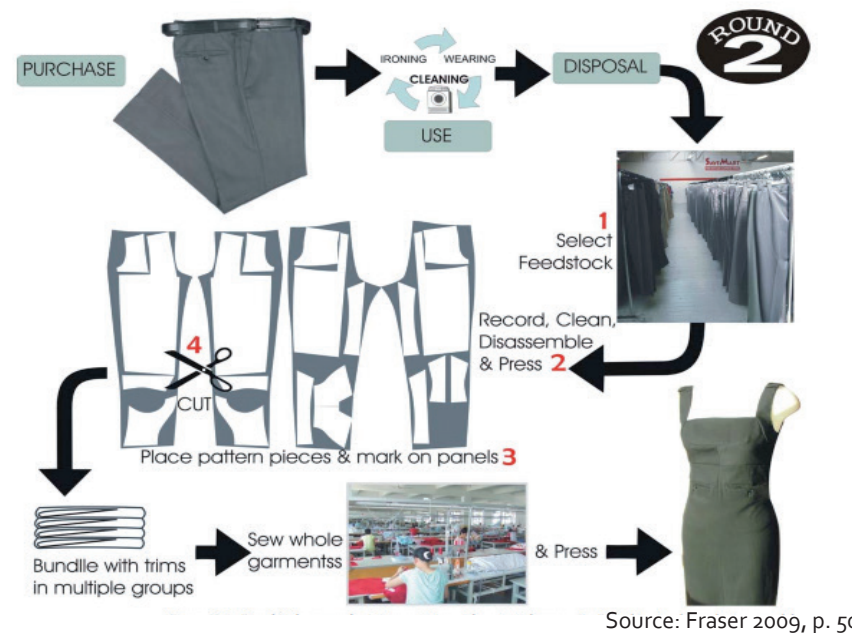
Fig. 9: Standardised upcycling process model
