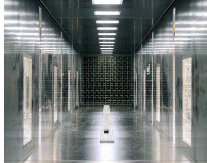
The 30-metre long wind tunnel, with its 3m x 3m active grid, is the scientific centrepiece of the Oldenburg WindLab.
