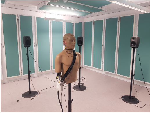
Fig. 5: Dummy head with inserted hearing device prototypes in a lab with variable acoustics. The green absorbing panels can be flipped to make them highly reflective.
