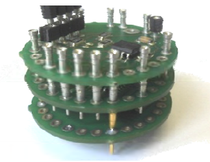
Figure 3. Stackable printed circuit boards exemplifying our approach to the modular design
