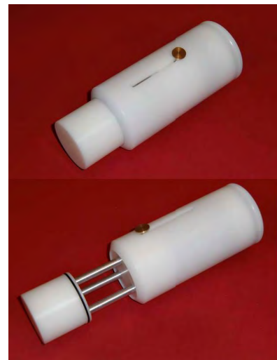
Figure 4. Construction of a protective cover for the deployed sensors shown in closed and open position
