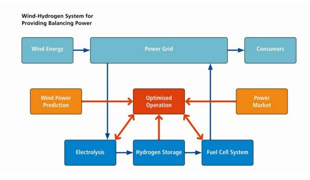
Figure 1: Principal structure of the HyWindBalance wind-hydrogen storage system.
