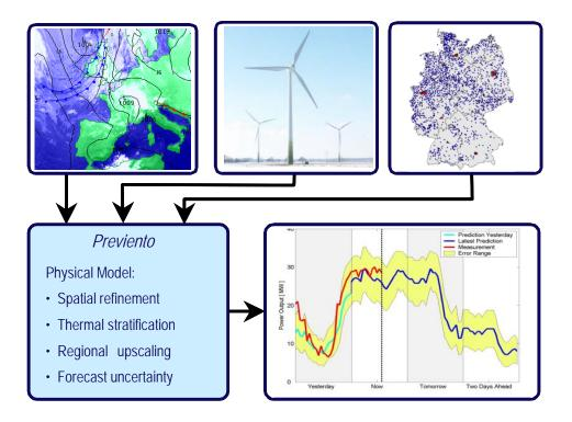
Figure 3: Basic scheme of the physical prediction system *Previento*. Based on weather data from several meteorological services and information on all German wind farms the system uses physical methods to provide a wind power forecast.
