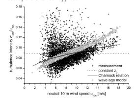
Figure 2: Measured and modelled turbulence intensities at 10 m height at Rødsand versus 10m wind speed
