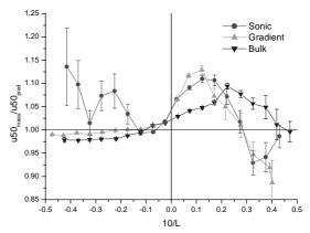
Figure 5: Comparison of different methods to determine the atmospheric stability; ratios of measured and calculated wind speeds at 50m height versus atmospheric stability are shown
