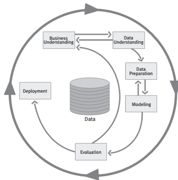
Figure 4.4: Phases of the CRISP-DM reference model 4
